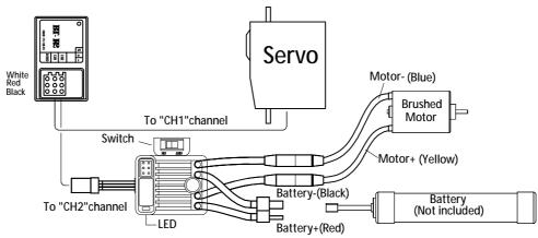
1. Connect the ESC, motor, receiver, battery and servo according to the diagram above. Pay careful attention to the polarities of all plugs and cables. If the polarity of the battery is reversed, the ESC can become permanently damaged. The polarity of the motor cables may be switched, this will reverse the direction in which the motor rotates.
